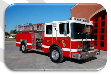
Type I engines must be capable of carrying at least four firefighters. The National Fire Protection Association's (NFPA 1901) standards require that all firefighters be carried in an enclosed cab. Designs of these engines have a crew cab capable of carrying 4 to 6 firefighters.
