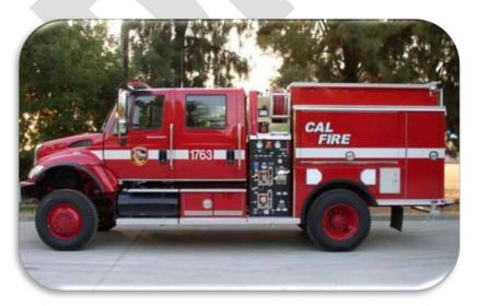
All CAL FIRE owned Engines are Type III. In addition to the standards above, they also carry a minimum of 500' of 3" hose used for supply and master stream operations. All engines are complimented with Basic Life Support medical equipment.
